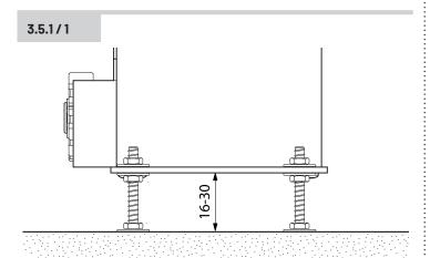
The height of the motor unit can be adjusted using the heavy-duty wall plugs.
